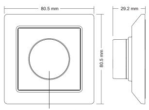
Click the rotary knob to switch ON/OFF paired Zigbee light devices
