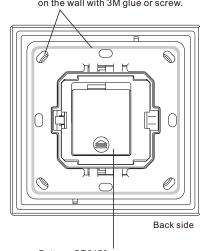
Battery: CR2450 Before the first use, please open the battery cover and remove the protective film
